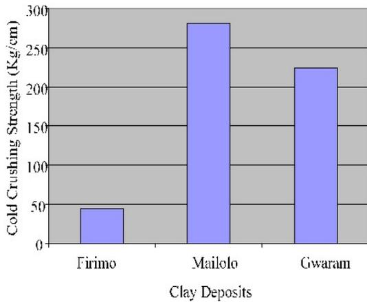
Figure 1: Cold Crushing Strength of the clays
