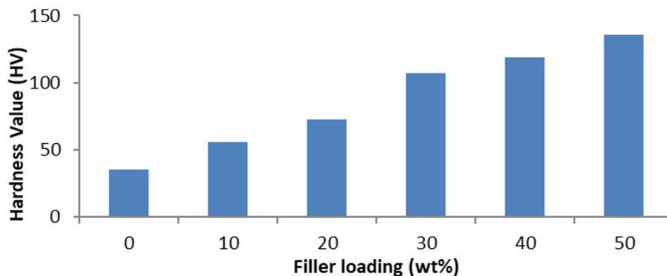
Figure 1: Variation of hardness value with the addition of SBAP
