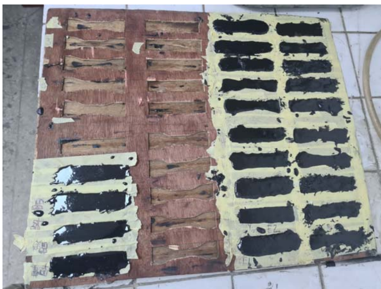
Plate 1: The Sample Composite In The Mold
