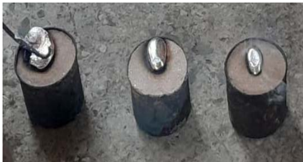
Plate 2: Cast samples in binder/sand formulations.
