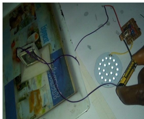
Figure 21. Miniaturized (25 by 25 by 4 mm) 1.4 V zinc-air cell Zn – air in series with a primary cell powering a lamp
