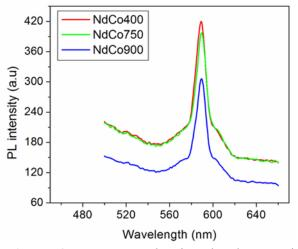
**Figure 6.** PL spectra showing the decrease in peak intensity as T<sub>A</sub> is increased. e<sup>-</sup>- h<sup>+</sup> recombination may take longer for NdCo900.
