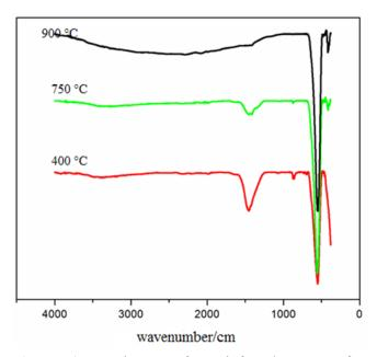
**Figure 4.** Fourier transform infrared spectra for NdCo400, NdCo750 and NdCo900 showing the reduction in peak intensity at 1400 cm<sup>-1</sup> and an increase in peak intensity at 600 cm<sup>-1</sup> with increase in annealing temperature.
