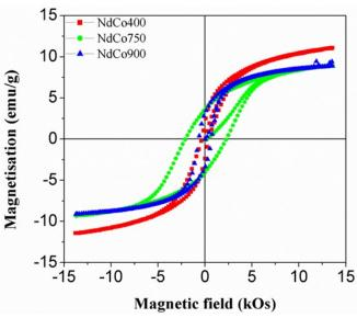
**Figure 5.** Room temperature magnetization hysteresis loops showing a decrease in saturation magnetization and increase in coercive field for powders annealed at 750 and 900°C.
