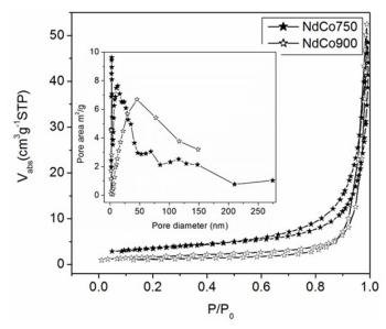
**Figure 3.** Adsorption-desorption isotherms for powders annealed at T<sub>A</sub> 750 and 900°C. The inset shows the disappearance of modal mesopore peaks as T<sub>A</sub> increased
