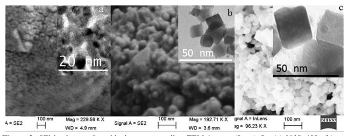
**Figure 2**. SEM micrographs with the corresponding TEM images (Inset) for (a) NdCo400, (b) NdCo750 and (c) NdCo900 showing the increase in crystallite size as T<sub>A</sub> increases
