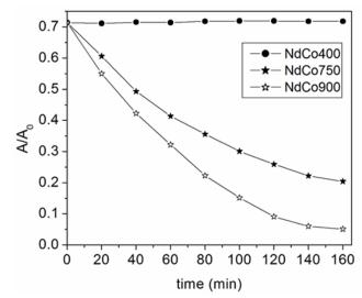
**Figure 7.** Photodegradation of RhB when irradiated with visible light for the photocatalysts NdCo400, 750 and 900 (1.5 g dm<sup>-1</sup>) in the presence of  $H_2O_2$  (3.0 × 10<sup>-5</sup> mol dm<sup>-3</sup>).
