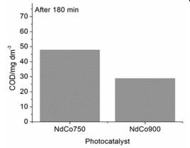
**Figure 8.** Analysis of the chemical oxygen demand (COD) for NdC750 and NdCo900 after a period of 3 hours of photodegradation. The mineralization efficiency is 54 and 73 % respective-
