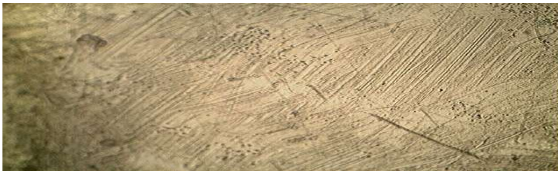
Figure 8: Photomicrograph of Pure Polyester Composite Sample with 200X magnification
