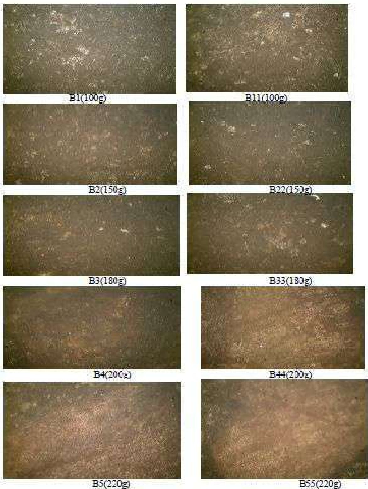
Figure 6:- Photomicrograph for 1.18mm particle size with 200X magnification
