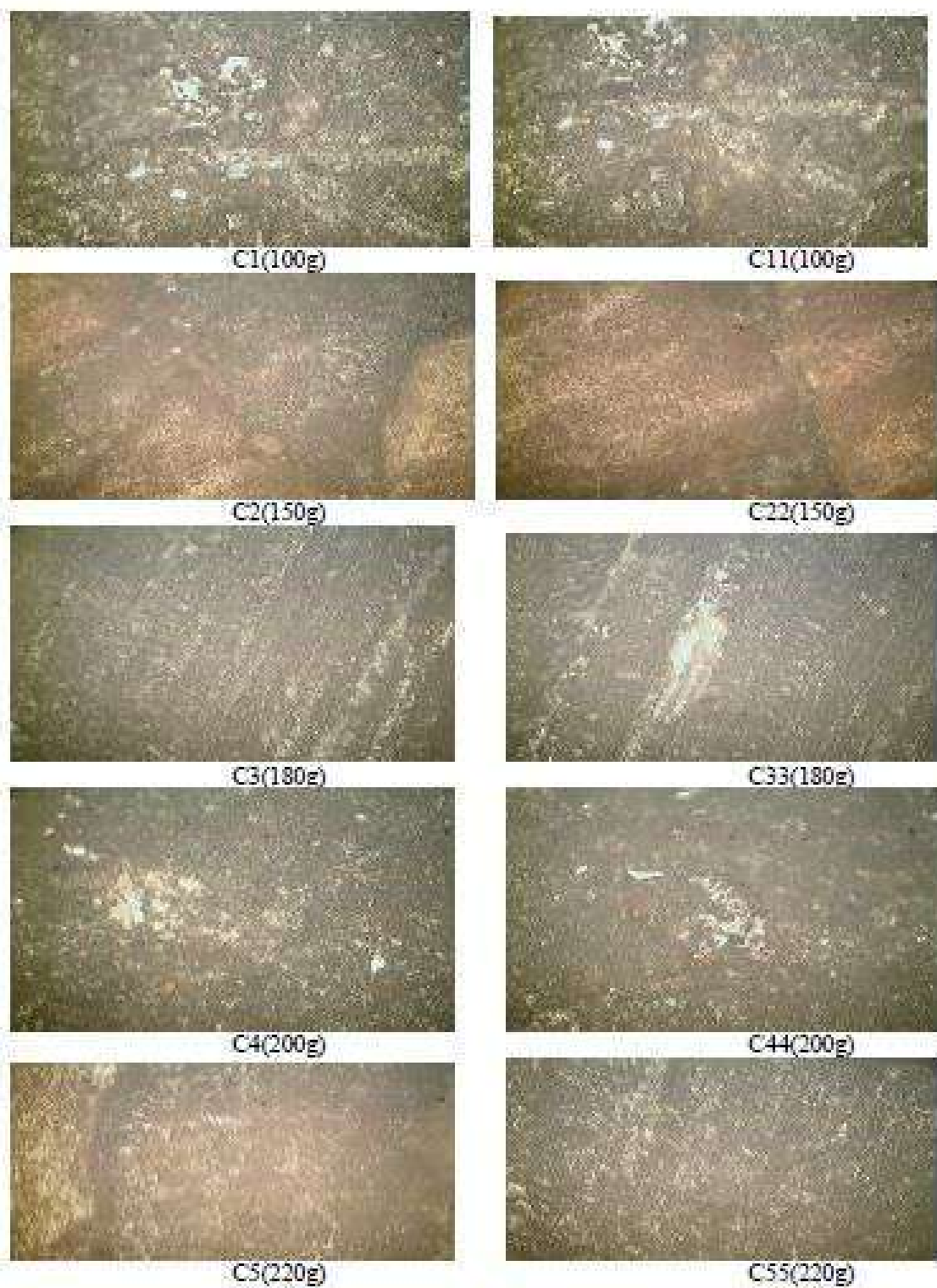
Figure 7: Photomicrograph for 2.36mm particle size with 200X magnification
