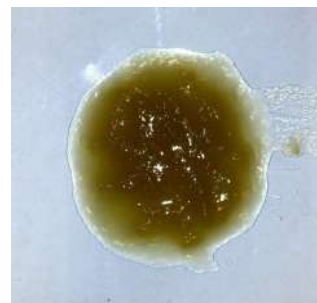
Figure 3: Photograph of Polymerized oil after 84 Days at 150°C in Ageing Vessel
