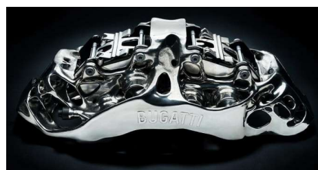
Figure 13: 3D Printed Bugatti 8-piston functional monobloc brake caliper produced with titanium
