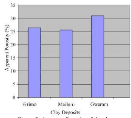
Figure 2: Apparent Porosity of the clays
