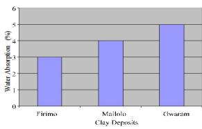
Figure 6: Water Absorption of the clays
