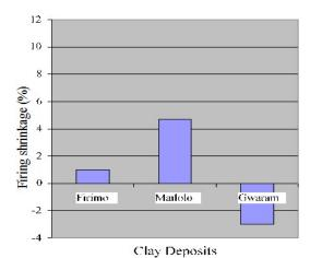
Figure 4: Firing Shrinkage of the clays
