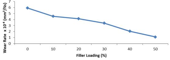
Figure 2: Effect of SBAP on wear behaviour of PP/SBAP composite
