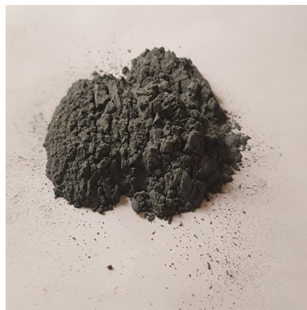
Figure 1: Silicon carbide particles of 25 µm size
