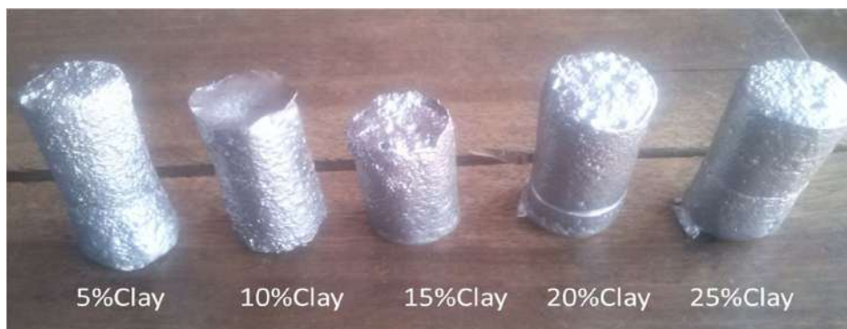
Plate 2: Surface appearance of Aluminum ingots casted from the blended sand.
