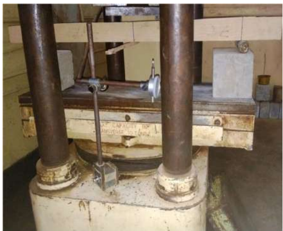
Plate 1: Laboratory Arrangement of the Three Point set up
