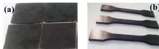
Figure 2: Prepared composites sheets (a) and cut samples for some mechanical tests (b)
