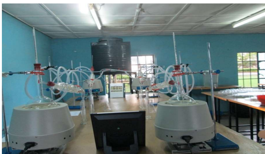
Plate I: Automated Coolant Recycling Distillation System
