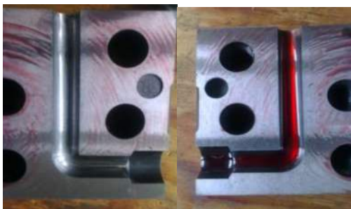
Figure 1: ECAE mould showing well-lubricated channels
