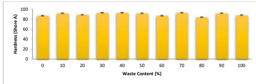
Figure 4: Hardness of Virgin/Waste LDPE blends different compositions
