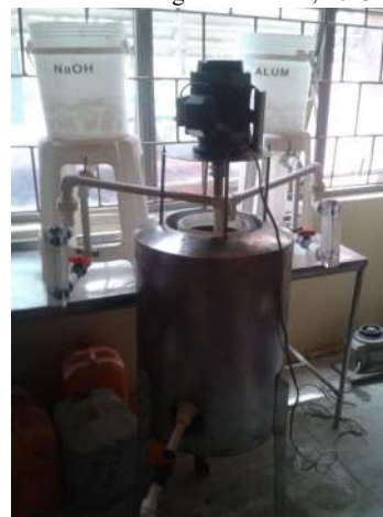
Plate I: Fabricated pilot scale reactor for the production of aluminium hydroxide from alum from Kankara kaolin.
